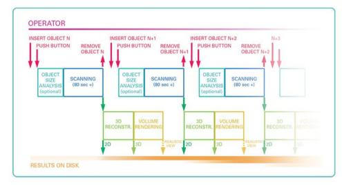
The pushbutton operating sequence doesn't require from the operator any interaction with keyboard or mouse and can be repeated multiple times. The reconstruction and visualization parts of the cycle run during scanning of the next sample. The sequence can be flexibly configured in advance for reconstruction and visualization parameters based on a predefined protocol or by repeating the reconstruction with the last selected settings.
