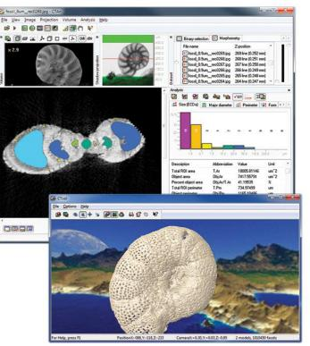
The CTAn / CTVol programs can create and visualize triangulated models of object surfaces. Such models can be saved in STL- file format. The STL-files can be sent to a 3D printer to build a magnified physical copy of the scanned objects using different materials. By selecting of volume of interest in CTAn, the physical model may be partially opened to get access to internal object details.
