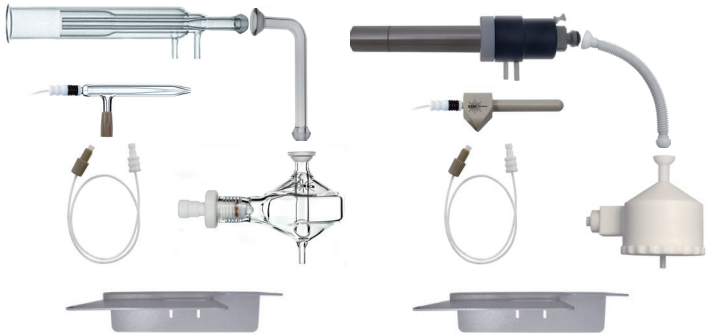
Aqueous sample introduction system, SeaSpray DC Nebulizer, Twister spray chamber, glass elbow and single piece quartz torch for Spectro Arcos EOP ICP-OES. Also required is mounting bracket for Niagara Rapid Rinse. HF-resistant sample introduction system, DuraMist DC Nebulizer, Tracey TFE spray chamber, PuraFlex transfer tube, and fully ceramic D-Torch for Spectro Arcos EOP ICP-OES. Also required is mounting bracket for Niagara Rapid Rinse.
