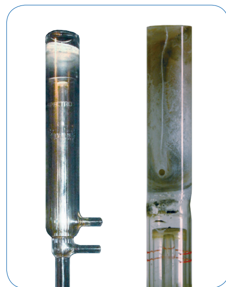
Figure 3: Examples of devitrification of quartz torches
