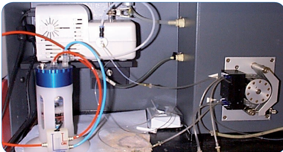
Figure 1: Experimental setup for the Varian Vista Radial ICP-OES with a Glass Expansion IsoMist Programmable Temperature Spray Chamber and the Capricorn Argon Humidifier attached.
