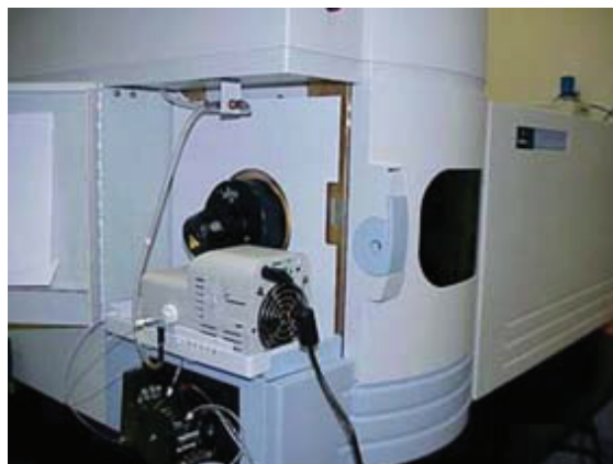
Figure 3. IsoMist mounted on the Optima 2100DV
