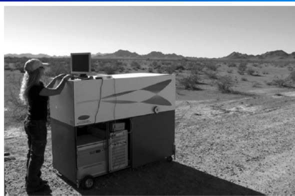
Fig. 4 Snapshot of the system during a field test of the stand-off LIBS sensor featuring C. López-Moreno.
