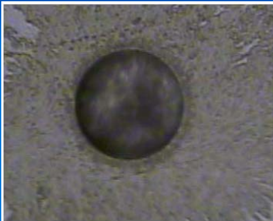
Figure 1: Image of 100um Quartz Sample after 500 shots at 10 Hz
