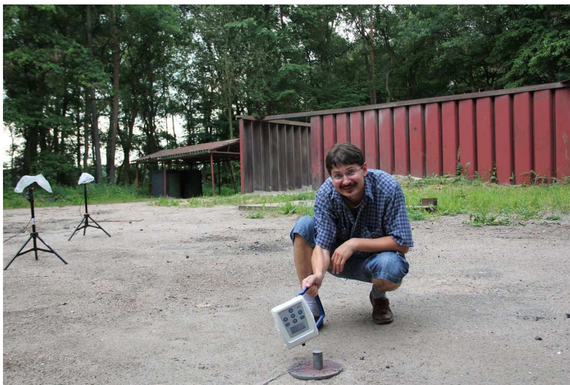
Figure 4. Practical application sampling of post blast traces of TATP in area of University of Pardubice, Institute of Energetic Materials
