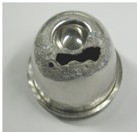
a) b) Figure 2. Phase diagram of Sn-Pb alloy and image of a ruined crucible.
