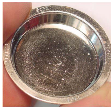
Fig 2. Example of mold imperfections on an old mold
