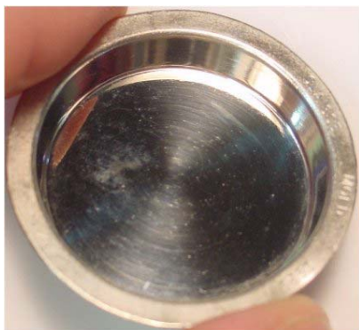
Fig 1. Example of mold imperfections on a recent mold
