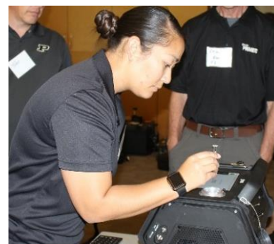
Figure 3-3 Sample Introduction via Syringe - Griffin G-510
