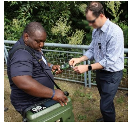
Figure 4-6 Hapsite ER Pine Needle Vapor Analysis
