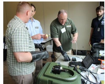
Figure 4-5 Operation of the Hapsite ER with PPE
