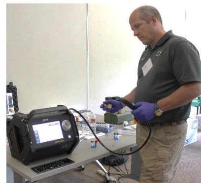
Figure 4-1 Griffin G-510 Operation in Vapor Sampling Mode
