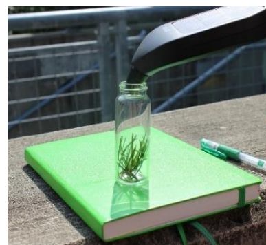
Figure 3-5 Analysis of Pine Needle Vapors - Griffin G-510
